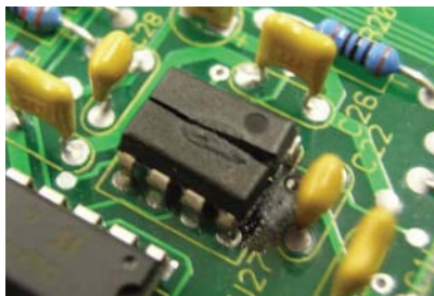
Figure 1 An EOS event can cause both the die and the package material to melt.
