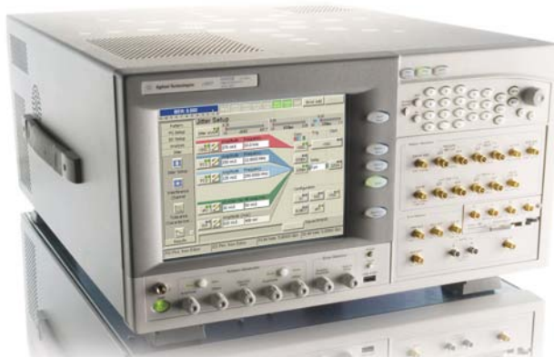
The N4903B high-performance serial jitter/bit-error-ratio tester is at the heart of the manufacturer's new test set for characterizing and analyzing conformance of hardware for implementing the new 8 billion-transfer/sec PCIe 3.0 serial bus, which owes part of its speed to use of 128/130-bit error-correction coding instead of 8/10-bit coding.
